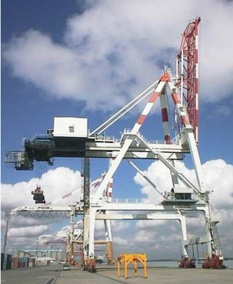
Image 36: This is the first Brisbane crane. Initially it was installed at Hamilton in the Brisbane river and later transferred downstream to be the first on the new Fisherman Island berths. It was a twin lift unit using the Callow System.
