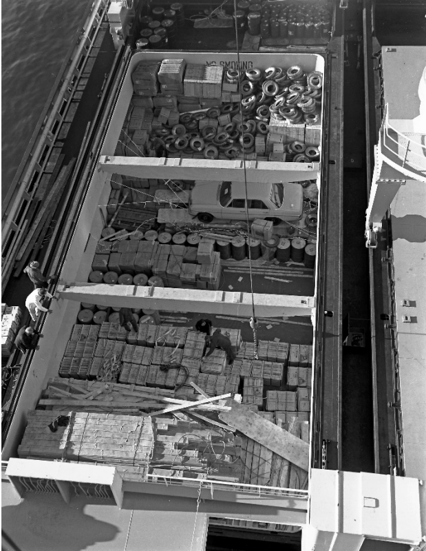
Image 1: This image illustrates break bulk, which means miscellaneous dry cargo in the hold of the vessel Atrevida in Fremantle harbour in May 1968. Each piece was man-handled individually into a rope net sling or to a crane hook to get it on or off the ship.
