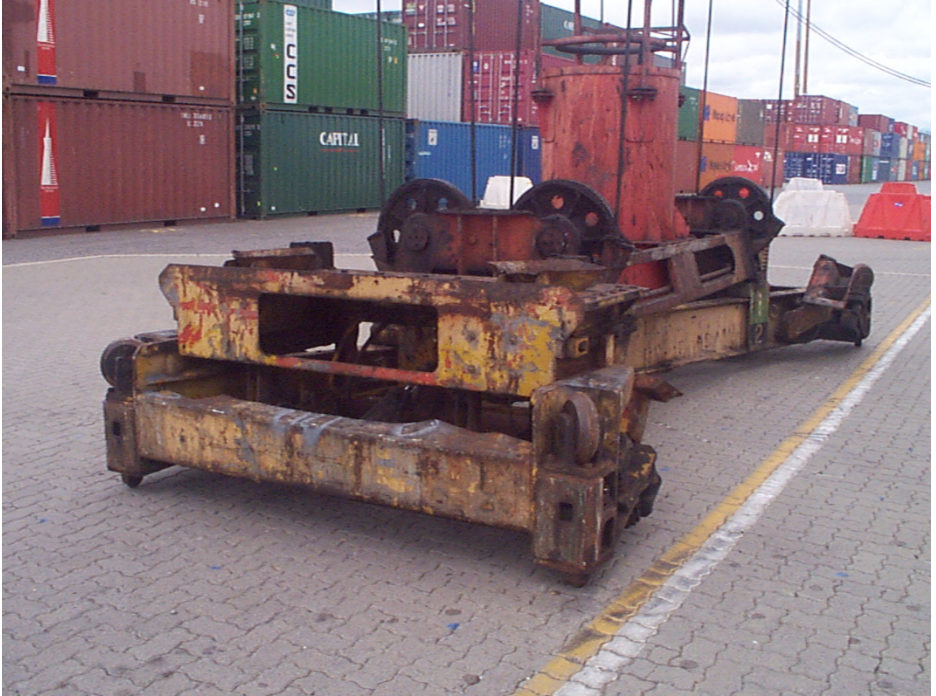
Image 39: Another view to illustrate the consequences of working ship cells.
