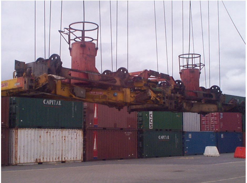
Image 37: This and the two images that follow show twinlift spreaders after 35 years service. The two central tubs collect and coil the multicore power cables that were suspended from the trolley above. These units handled the ISO 20 ft containers and are fitted with twist locks for connection to them.
