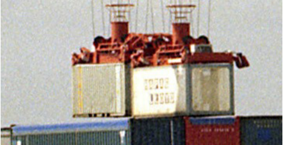
Image 33: This enlarged view of the twin lifting spreaders shows that the twin lifted containers are of different heights, and are lifted by spreaders set at different levels. This was not noticed by the crane driver, the crane or the ship. It was routine. No modern twinlift crane can match this.
