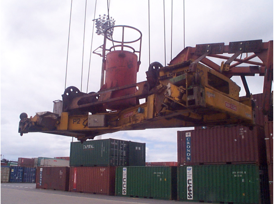
Image 38: This shows the light construction of these spreaders and head blocks.
